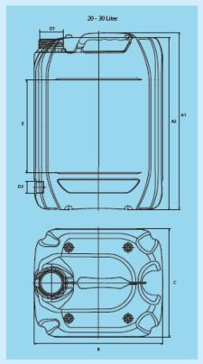
A 1 = overall height A 2 = stack height B/C = base area D 1 = outlet diameter
